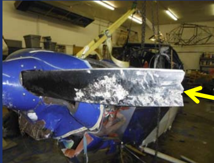
.30 Caliber Bullet hole that was improperly repaired by previous owner
